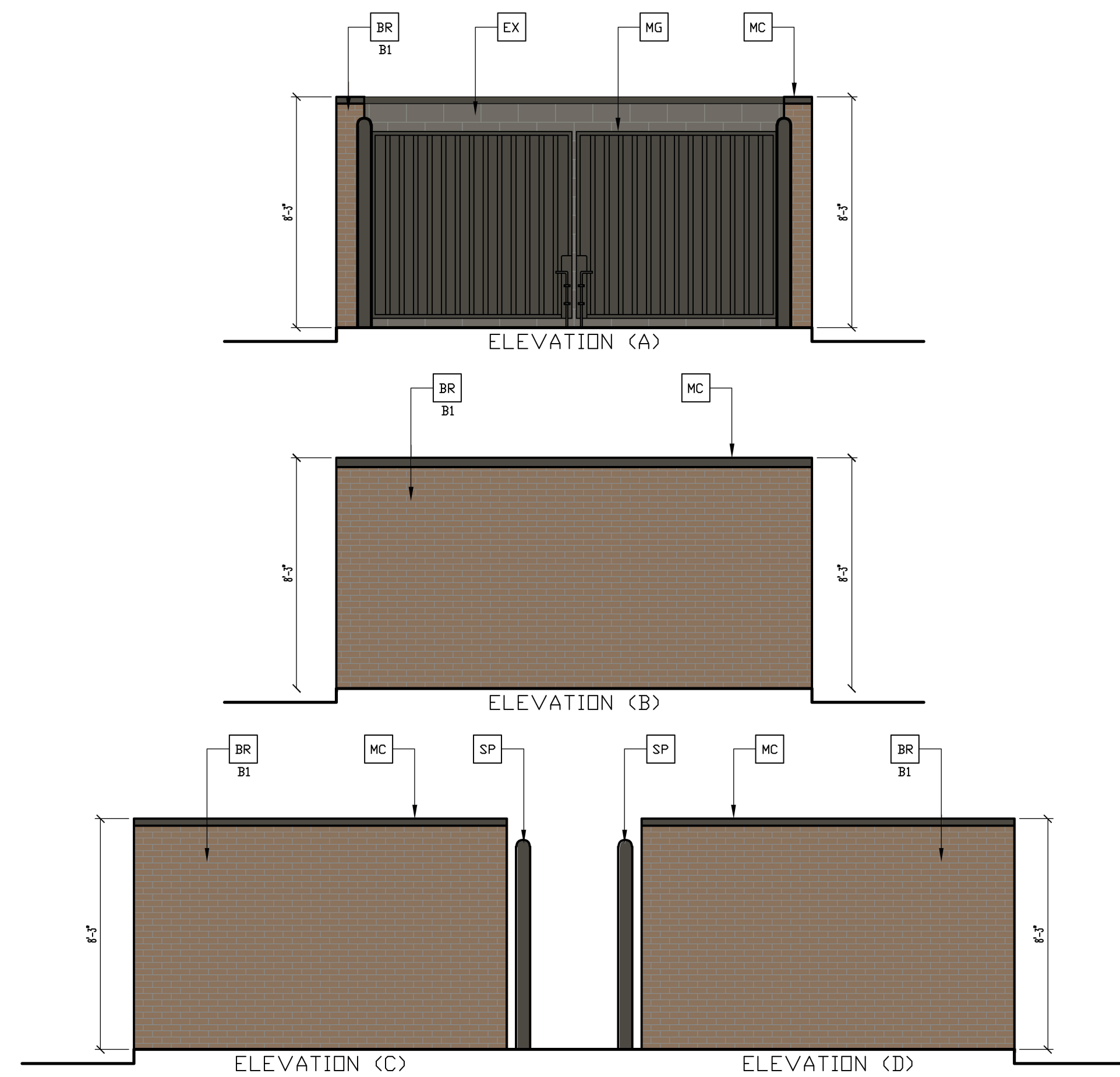
2 DUMPSTER ELEVATIONS SCALE 1/4"=1'-0"
